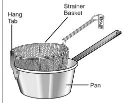
warning: Always remove the strainer basket **SLOWLY** from pan to allow hot liquid to drain. Lifting strainer basket out of pan too quickly will cause hot liquid to spray out of basket and could result in severe burns for anyone near the pan.
