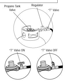
NOTE: Type 1 fittings are made with a metal to metal seal and must be made very tight to prevent leaking.
