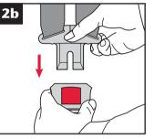
pushing them firmly until you hear a click (dia 2b). Make sure the harness is not twisted. Tighten the harness by pulling the adjuster strap forward making sure the harness is a comfortable but FIRM fit around your child (dia 2c). **IMPORTANT** – The lap section of the harness should rest as
