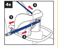
(dia 4e). Check that the child seat feels secure and that the seat belt is not twisted.
