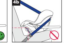
vehicle is not suitable for use with the alternative routing (dia 4c). The lap section of the seat belt should pass through both belt quides underneath the foot end of the seat.
