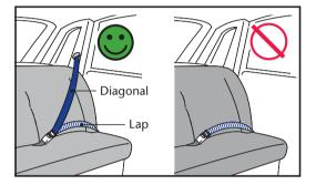
**IMPORTANT** – The child seat **MUST** only be used with a lap and diagonal seat belt (approved to UN/ ECE Regulation no. 16 or other equivalent standards).
