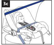
back of the car and move the handle to the stable position as shown, making sure it is latched properly (dia 3b). Fasten the seat belt across the child seat. Pass the lap section of the seat belt through the lap guides on both sides as indicated by the blue arrows on the child seat. Pull the diagonal section of the seat belt around the back of
