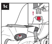
Place your child in the child seat and check that the shoulder strap slots are level with, or just below, your child's shoulders and that the head is comfortably positioned in the head support when used (dia 1d). To adjust the height of the shoulder straps, first remove your child from the seat. Remove the shoulder pads (if applicable) by sliding them off the shoulder straps. Next, pull one strap through
