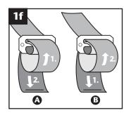
The adjuster at the end of the crotch strap is found under the front edge of the child seat. To change the length of the crotch strap, thread it through the adjuster in the direction of the arrows shown (dia 1f). A – Shortening
