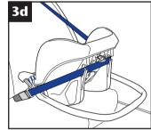
Feed the diagonal belt through both diagonal belt guides indicated by the blue arrows at the back of the seat (dia 3d). Tighten the seat belt by first pulling at **1** and then **2** and 3 to remove any slack (dia 3e). Check that the child seat feels secure and that the seat belt is not twisted. **IMPORTANT** – If your car
