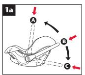
Handle – carrying, rocking and stable position To move the handle, push firmly in towards the shell to release lock and then move it to the desired position (dia 1a): A – Carrying position Rocking position **G** – Stable position
