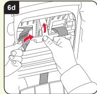
Push the chest pad strap through the shoulder strap slot towards the back of the seat. Attach the chest pad strap to the chest
