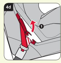
Whilst holding the diagonal belt tight pull up on the clamp lever **1** until it engages (dia 4d).
