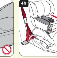
The child seat should now be secure. To check pull forward firmly on the harness. There should be little or no movement (dia 4h).
