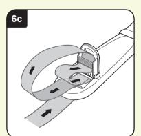
Feed the harness strap under the SAFESTRAP<sup>™</sup> mechanism. Push through the harness strap until it appears out the top of the chest pad. Ensure the strap is not pad adjustment arm (dia 6d). twisted (dia 6c).
