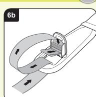
Making sure the harness strap is not twisted Ensure there is enough slack and thread push the loop end of the harness strap up through the front of the SAFESTRAP™ mechanism and pull through (dia 6a).
