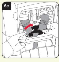
Push the harness strap through the shoulder strap slot towards the back of the seat. Attach the harness strap to the yoke. Ensure the harness strap and the chest pad strap are not twisted (dia 6e).
