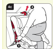
**IMPORTANT** – Do not twist the belt Firmly push the child seat into your vehicle seat using your body weight. Pull and hold the diagonal belt **1**. Pull at **2** to remove all **IMPORTANT** – Do not twist the belt.
