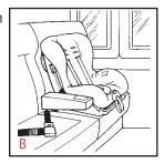
WARNING: WHEN USING THE RESTRAINT IN FORWARD FACING MODE, ATTACH THE VERSA-TETHER ONLY TO TETHER ANCHORS IDENTIFIED BY THE VEHICLE MANUFACTURER AS TETHER ANCHORAGE POINTS. USE OF OTHER LOCATIONS IS NOT APPROVED OR PERMITTED.
