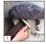
If there is a problem stabilizing the child restraint, place a rolled towel in the crease of the vehicle seat to help level the child restraint base.
