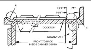
Refer to the cooktop installation instructions for dimensions of cooktop, countertop cut-out, and cabinet requirements. The RMDD3004 can be installed in most standard 30" wide cabinets, (RMDD3604 can be installed in most standard 36" wide cabinets), (RMDD4804 can be installed in most standard 48" wide cabinets).
