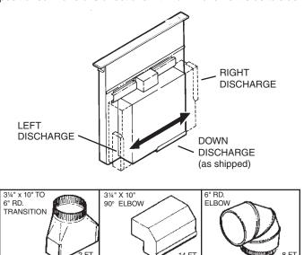
The system will operate most efficiently when the ductwork does not exceed 40 feet of equivalent duct. The chart above, shows equivalent feet of elbows and transitions. The number of feet of straight  $3\frac{1}{4}$ " x 10" or 6" duct plus the equivalent feet of elbows or transitions to be used should equal 40 feet or less.
