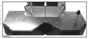
**7.2.2** Press the metal shutoff plate on a surface to completely flatten bent flange and install on the top of the blower, using the 3 screws previously set aside plus another no. 8 x 1/2" screw (from parts bag).
