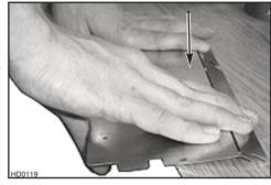
**7.2.3** Fold down the foldable flange of the adapter/damper. This flange must be at 90° from the remaining flanges. See picture beside.
