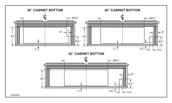
See figures below for cut-out dimensions for ducting.
