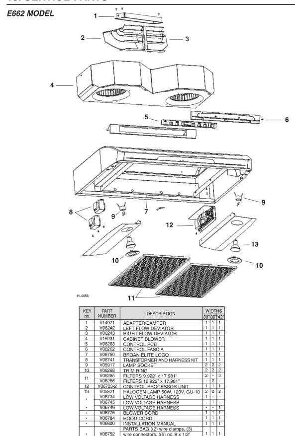
wire connectors, ((5) no. 8 x 1/2 screws, (9) no. 8 x 3/8" screws)
