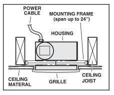
Housing mounted anywhere between <u>trusses</u> using mounting frame.
