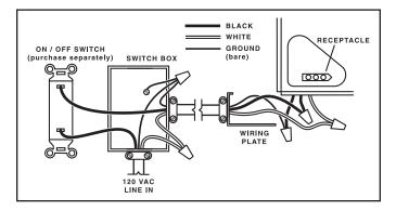
5. Run 120 VAC housing wiring to installation location. Use a UL approved connector to secure house wiring to wiring plate. Connect wires as shown in wiring diagrams.
