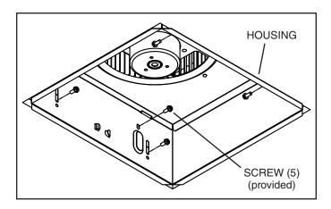
7. Position the two movable brackets of the mounting frame directly across from each other and insert the housing into the mounting frame until it touches the duct connector bracket. Secure the housing to the mounting frame and duct connector bracket using the (5) screws provided.
