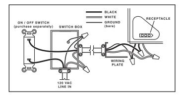
Retrieve the existing electrical wiring from above the ceiling and use a UL approved connector to secure it to the wiring plate. Re-attach wiring plate to fan housing, if necessary. Connect wires as shown in wiring diagrams.
