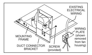
5. Attach the duct connector bracket to the mounting frame using the (1) screw provided. Position the bottom edge of the duct connector bracket so it touches the finished surface of the ceiling and tighten the screw.
