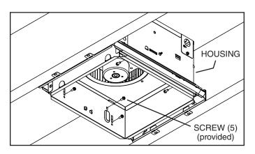
3. Position the two movable brackets of the mounting frame directly across from each other and insert the housing into the mounting frame until it touches the duct connector bracket. Secure the housing to the mounting frame and duct connector bracket using the (5) screws provided. Position the housing horizontally as desired.
