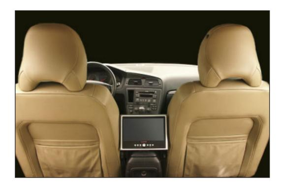
Brodit offers an easy-to-use system for mounting multimedia monitors in the vehicle. It is based on a car specific mount with a monitor mount. The monitor will be placed between the front seats, giving the back seat passangers a perfect view.
