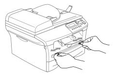
2 Using both hands put the one sheet of paper in the manual feed slot until you feel the front edge of the paper touch the paper feed roller. Let go of the paper when you feel the machine feed the paper in a short distance.
