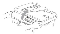
You can still use the DCP while the scanner cover is up. To close the scanner cover, push it down with both hands.
