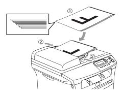
3 Unfold the ADF document output support flap.
