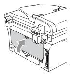
7 Put the drum unit and toner cartridge assembly back into the DCP.
