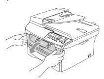
2 Pull out the drum unit and toner cartridge assembly.
