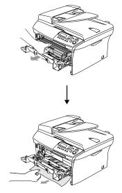
5 If you can not remove the drum unit and toner cartridge assembly easily, do not use extra force. Instead, lift the scanner cover and use both hands to carefully pull the jammed paper up and out of the output tray opening.
