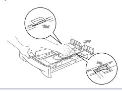
3 Fan the stack of paper well to avoid paper jams and mis-feeds.
