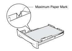
5 Put the paper tray firmly back in the DCP and unfold the output paper tray support flap before you use the DCP.
