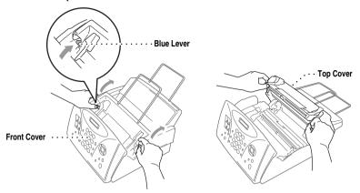
3 Pull the jammed paper gently from the paper feeder toward the back of the fax machine. If the paper remains jammed, then pull it toward the front of the machine.
