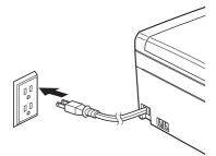
Connect the telephone line cord. Connect one end of the telephone line cord to the jack on the machine marked **LINE** and the other end to a modular wall jack.
