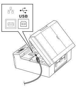
C Carefully guide the USB cable into the cable channel and out the back of the machine. Connect the cable to your computer.
