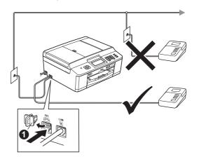
Set the receive mode to External TAD if you have an external answering machine. See Choose the correct Receive Mode on page 9. For additional details, see Connecting an external TAD (telephone answering device) in chapter 6 of the Basic User's Guide.
