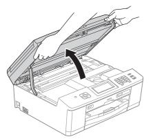
Connect the USB cable to the USB socket marked with a e symbol. You will find the USB socket inside the machine on the right as shown below.
