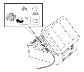
C Carefully guide the network cable into the cable channel and out the back of the machine. Connect the cable to your network.
