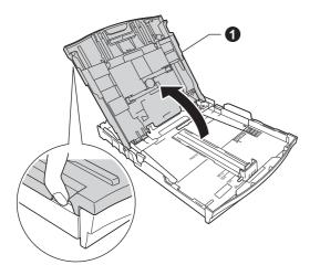
C With both hands, gently press and slide the paper side guides ● and then the paper length guide ② to fit the paper size.
