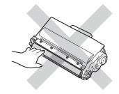
Put the new toner cartridge firmly into the drum unit until you hear it lock into place. If you put it in correctly, the green lock lever on the drum unit will lift automatically.
