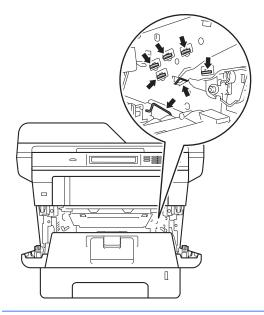
4 Push down the green lock lever and take the toner cartridge out of the drum unit.
