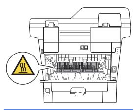
Using both hands, gently pull the jammed paper out of the back of the machine.
