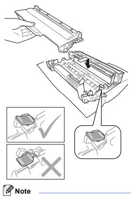
Make sure that you put in the toner cartridge correctly or it may separate from the drum unit. 8 Put the drum unit and toner cartridge assembly back into the machine.
