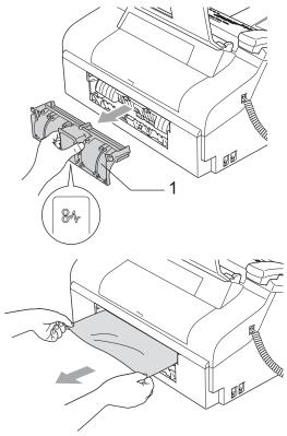
Put the Lower Jam Clear Cover back on. Make sure the cover is set properly.
