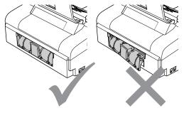
5 Open the Upper Jam Clear Cover (1). Make sure that there is no jammed paper left in the corners of the machine.
