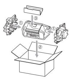
8 Pack the printed materials and additional parts in the original carton as shown below. Do NOT pack the used ink cartridges in the carton.
