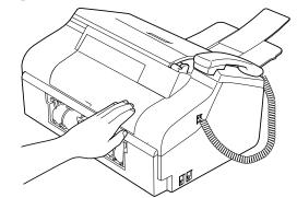
Push the paper tray firmly back into the machine. While holding the paper tray in place, pull out the paper support until it clicks and unfold the paper support (See the illustrations in *Loading paper* on page 10).
