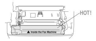
1 Open the top cover. Make sure the top cover is completely open. To remove the drum unit, hold each side of the drum by its handles and gently lift the drum forward toward you.
