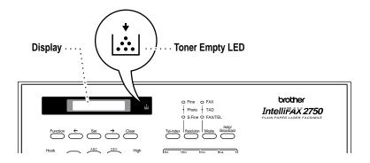
The Toner Empty LED light stays on and the display shows TONER EMPTY to indicate that the toner is empty. Once this indication appears, your fax machine will not resume printing until you have installed a new toner cartridge.
