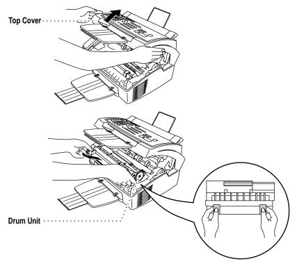
Place the drum unit on a drop cloth or large piece of disposable paper to avoid spilling and scattering the toner.
