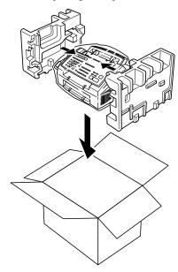
Place documents (manual and printed material) and the drum unit and toner cartridge assembly into the original carton as shown below:
