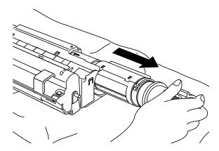
4 Unpack the new toner cartridge. Place the used toner cartridge into the aluminum bag and discard it according to local regulations.
