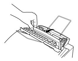
2 Fan the paper well. Load the paper, making sure that the print side is toward the fax machine and the paper level is stacked below the paper mark. The feeder can hold up to 200 sheets of paper, or up to 10 envelopes.
