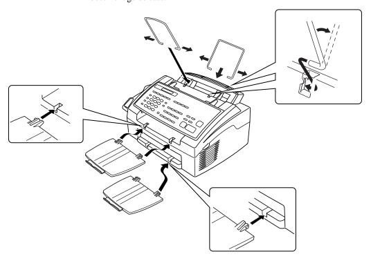
**5** Attach the document and paper trays to the fax machine and pull out their extensions.
