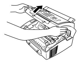
**3** Holding the drum unit by its handles, insert it into the fax machine.
