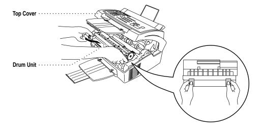
**3** Remove the toner cartridge from the drum unit and keep it in a safe place. For more information, see "Replacing the Toner Cartridge" on pages 112–116.
