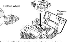
Make sure that the end of the tape feeds under the tape guides. • If the ink ribbon is loose, use your finger to wind the toothed wheel in the direction of the arrow on the cassette After you have installed the tape, feed the tape (see Feeding) once and then push
