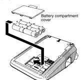
Attach the battery compartment cover by inserting the three hooks at the ottom into the slots on the machine, then pushing down firmly on the cover until it snaps into place.
