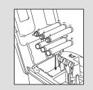
When using the P-touch labeler with batteries, insert six new AA alkaline batteries (LR6), making sure that their poles point in the correct directions. Always replace all six batteries at the same time using brand new ones.
