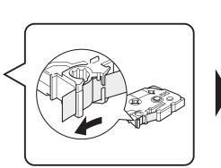
Make sure that the end of the tape feeds under the tape guides.
