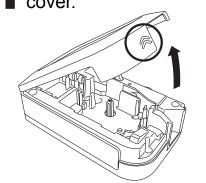
Verify that the P-touch labeler is turned off. Open the cassette cover as shown by the arrow in the above illustration while pressing the part marked "<<".
