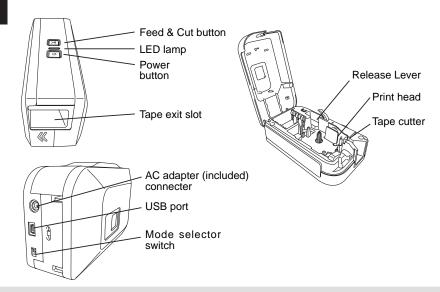
The PT-2430PC has 2 mode selector settings - "EL" and "E". The mode selector switch is pre-set at the factory to the EL mode, for use with P-touch Editor Lite. For E mode, you will need to install P-touch Editor 5.0, a more advanced labeling software, and the required drivers from the enclosed CD. For details on how to install the P-touch Editor 5.0, see "Starting P-touch Editor 5.0" below.
