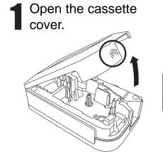
Verify that the P-touch labeler is turned off. Open the cassette cover as shown by the arrow in the above illustration while pressing the part marked "<<".
