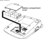
Attach the battery compartment cover by inserting the three hooks at the bottom into the slots on the machine, then pushing down firmly on the cover until it snaps into place.
