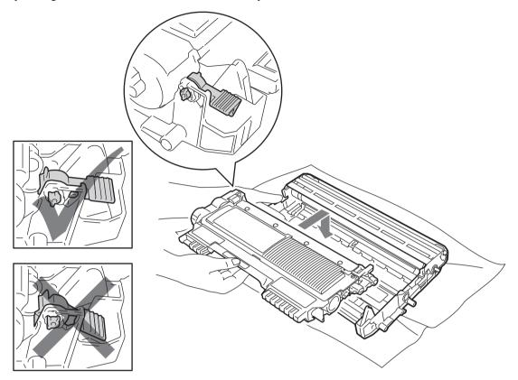
17 Open the front cover. Put the drum unit and toner cartridge assembly back into the machine.
