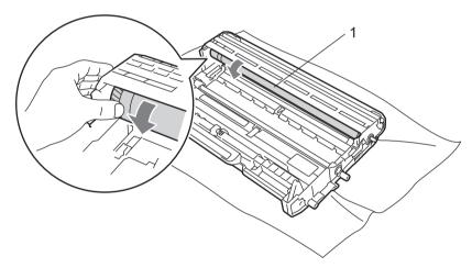
7 When you have found the mark on the drum that matches the print sample, wipe the surface of the OPC drum with a dry cotton swab until the dust or glue on the surface comes off.
