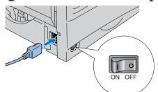
Make sure that the printer power switch is off. Connect the AC power cord to the printer. Do NOT connect the interface cable.
