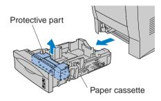
Pull out the paper cassette, and then remove the protective part from the
