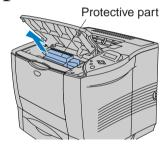
Remove the protective part from the printer.
