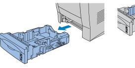
Pull the paper cassette completely out of the printer.
