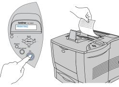
Press the Go switch. The printer prints a test page Check that the test page has printed correctly.
