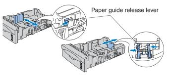
While pressing the paper guide release lever, slide the adjusters to fit the paper size. Check that they fit correctly into the slots.
