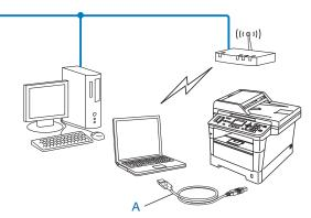
You can configure the wireless settings of the machine using a USB cable temporarily connected to a wired or wireless computer.
