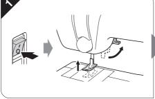
Stop the machine with the needle in the fabric at the
