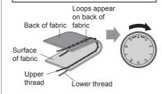
Solution: Increase the tension by turning the upper tension control dial to a higher number.
