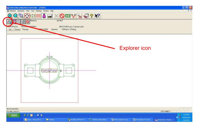
1. Left click on the drive or folder containing the DST file you want to read in. In this example the  $3\frac{1}{2}$  Floppy (A) is being used.
