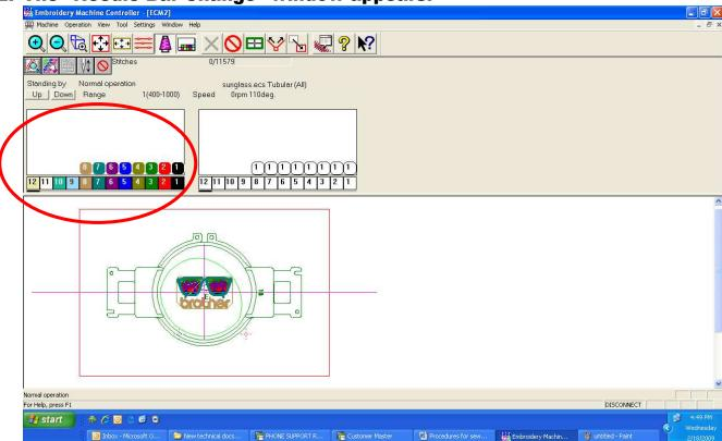
3. The bottom colors, of the Needle Bar Change window, (1-12) represent the 12 needles on the machine.
