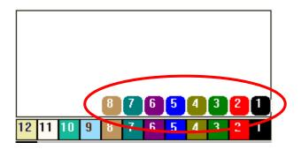
5. To select the 1<sup>st</sup> color of the design to sew needle 12, you click and drag the color change bubble over needle 12. When doing this, please make sure and keep the bubble within the color change window as indicated by the red dashed line or your change will not take effect.
