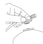
Check the rubber seal in the valve. Turn the valve clock-wise until the valve is firmly connected to the canister. Check for any leaks before igniting stove. Turn the butane canister counter-clockwise to disconnect the stove.
