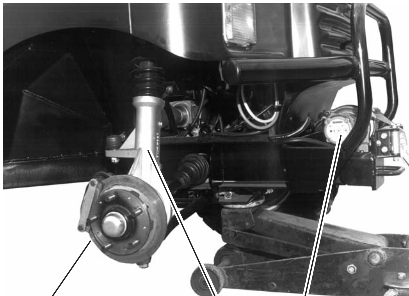
Disc Brake Assembly Front Strut Assembly Winch (Optional)
