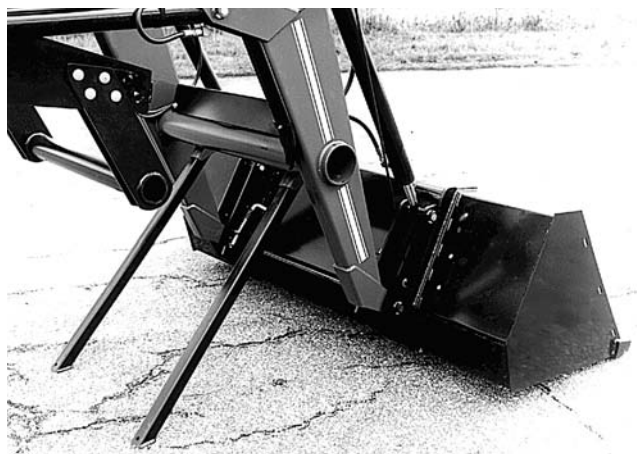
Figure 2-7 Parking Stands Installed
