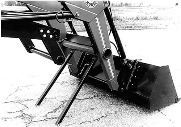
Figure 5-1 Parking Stands Installed
