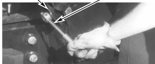
Figure 2-7 Clamp Installed In Working Position Tightening Quick Attach Nut Using Self Storing Tool
