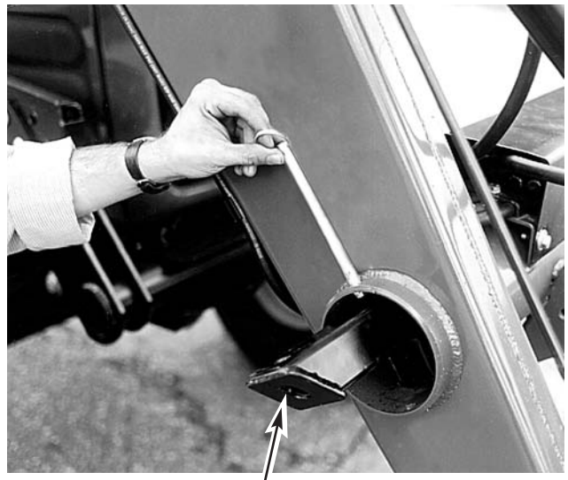
Fully Insert Stands And Pin Into Place
