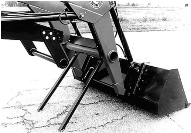
Figure 5-1 Parking Stands Installed
