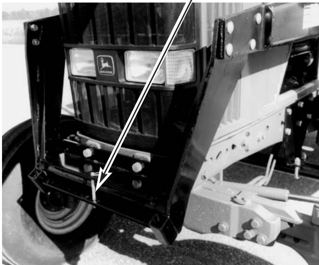
Figure 2-3 Front Bracket Pin
