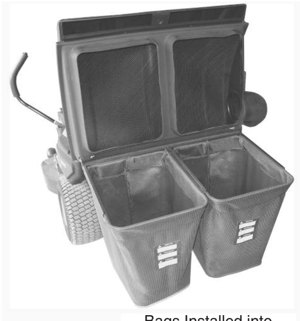
Bags Installed into Support Frame
