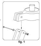
• Locate the *Finderscope (1)* with pre-assembled mounting bracket. Remove the two nuts located near the front of the telescope (closet to the eyepiece) and place the Finderscope and bracket assembly over the exposed screws. Replace the nuts, and securely tighten the Finderscope and bracket assembly in place.
