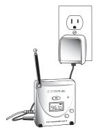
The FM Transmitter 2 will operate on the included AC Adapter. It will also operate on two "AA" size Alkaline batteries (optional).
