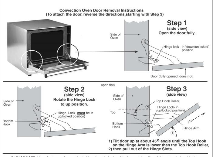
**PLEASE NOTE:** Hinge Locks may become jostled into the unlocked position by rough handling of the carton during shipping, causing the door to be unhinged from the oven when the carton is opened. If this occurs, follow the directions for attaching the door.
