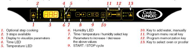
The Dynamic control panel can work both in Manual and in Programmed modes. For each cooking cycle (both in the Manual and in the Programmed mode) the operator can set 3 cooking steps. For each step, you enter cooking time, oven temperature, and humidity %.
