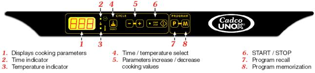
The Classic Control Panel can operate in "Manual" and in "Programmed" modes. For each cooking cycle (both in the Manual and in the Programmed mode) the operator can set cooking time and oven temperature.
