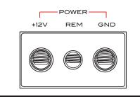
Before you begin with your installation, disconnect the NEGATIVE (-) terminal from your car's battery. This safety precaution will avoid possible short circuits while wiring your amplifier. Cadence amplifiers operate on 12-volt negative ground systems only.
