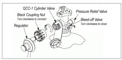
Place the dust cap on the cylinder valve outlet whenever the cylinder is not in use. Only install the type of dust cap on the cylinder valve outlet that is provided with the cylinder valve. Other types of caps or plugs may result in leakage of propane.
