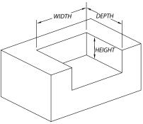
The drawings below show the different types of cabinet cut-out dimensions for side burners.
