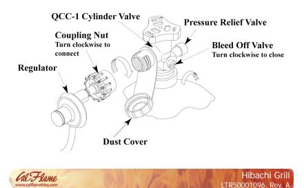
The maximum fuel capacity is 20 lbs. of propane, or 5 gallons. Full cylinder weight should be approximately 38 lbs. (43.7 lbs. nominal water capacity.) Never fill the cylinder beyond 80% full.
