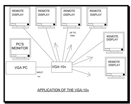
All connectors are on rear of case. Includes "Control" input and expansion output for tutor control of Autoswitch based classroom system. Turning the ControlSwitch (available from Calibre) On/Off enables/disables monitors connected via Calibre's AutoSwitch. Multiple VGA-10+s can be interlinked for large installations.
