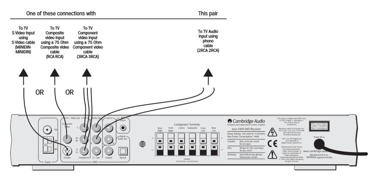
If your TV has S-Video inputs, an S-Video interconnect can be used to connect this player. When the S-Video output is used the component video outputs cannot be used.
