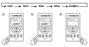
To select the option you require release the button when the menu option is displayed on the screen (Fig. 2).
