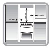
The height of the cooker can be adjusted by means of adjustable feet in the plinth (900mm - 930mm). Adjust the feet by tilting the cooker from the side. Then install the product into position.
