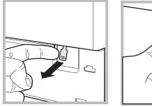
4. pull outwards using the tab as indicated in the figure, until the plastic tie-rod is freed from its stop position; pull downwards and open the door at the same time.5. reposition the panel, making sure the hooks are securely in place before you push it onto the appliance.
