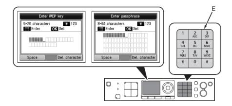
Press the  $\bigstar$  button to switch character entry modes. Network key entry is case-sensitive.
