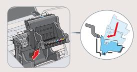
**5** Lower the lock lever and gently press it down until it locks into place.
