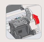
Gently slide the print head into the holder. The print head will rest at a slight angle. Do not press it down.
