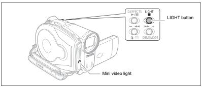
Set the camcorder to a recording mode ( CAMERA · '\) or CAMERA · C ) and press the LIGHT button.
