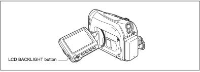
You can switch the brightness of the LCD screen between normal and bright by pressing the LCD BACKLIGHT button. This is useful for outdoor recordings.
