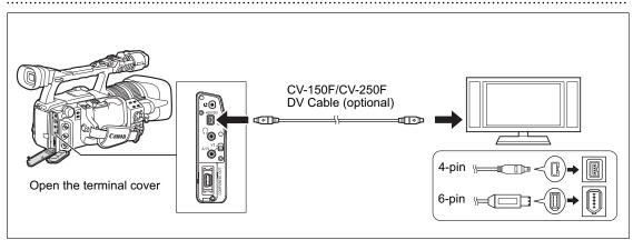
• When connecting the camcorder to a monitor TV that supports DV, you may need to carry out a procedure on the TV to recognize the camera. Refer to the instruction manual of the TV or monitor.
