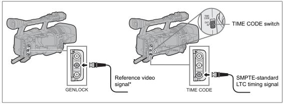
\* As a reference video signal input you can use either an HD Y signal or an NTSC composite video signal.
