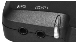
Use 1/P2 for remote manual flash
